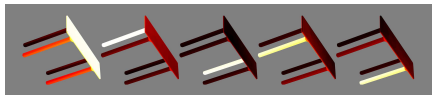
Fig. 4. NMF basis functions ( k = 5 ) for the table mesh. The table top and each leg are isolated in different functions.
