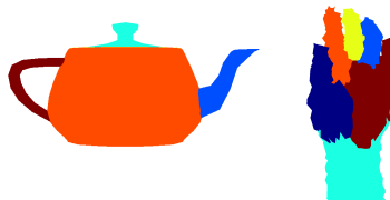
Fig. 11. The NMF segmentation method can handle meshes with multiple components and meshes that are not watertight, such as the teapot, k=4 (left) and noisy meshes, such as the hand, k=6 (right).
