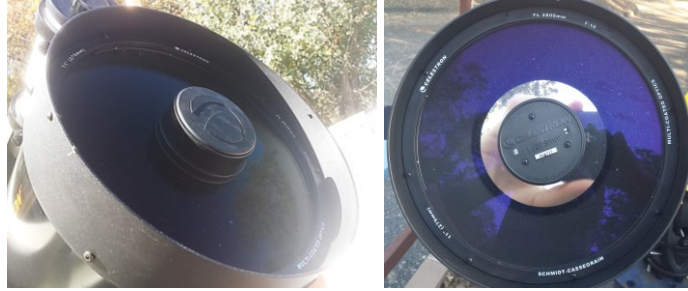
Figure 28. Two views of the aperture of the C11 captured by Foley. Note the optical obstruction caused by the corrector plate to which the secondary mirror is mounted internally. (In the image on the right, a cosmetic cap not affecting the aperture shape has been removed.)
