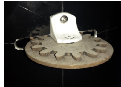
Figure 56. The method of mounting each gear from the outside. A bracket complementary to the white bracket visible here lies on the underside of the gear lip. The metal axle bridging them is surrounded by an unseen plastic bushing inside the gear–lip stack.
