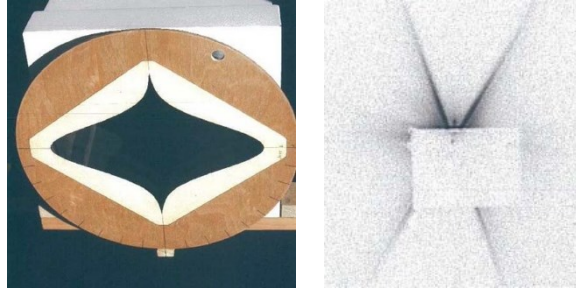
Figure 21. Left, the mask used by Daley to observe Sirius (Daley, 2014). Right, the corresponding CCD image recorded using this mask in tandem with a small “coronagraph focal mask foil” to reveal Sirius B (Daley, 2014).
