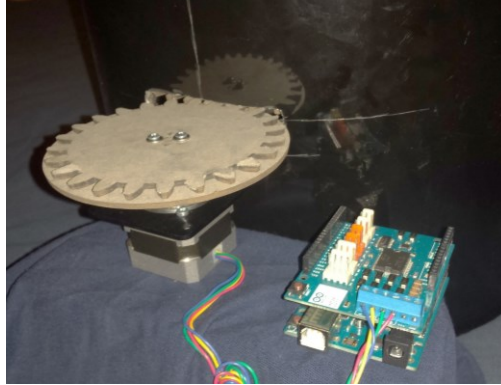
Figure 57. The size of the driving motor mandated a pinion larger than the guiding gears.
