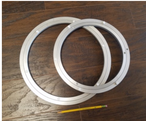
Figure 61. The bearings acquired in the process of evaluating the potential of the lazy Susan design. Pencil included for scale.
