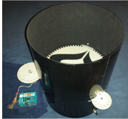
Figure 59. The virtual axis design seen with a mask. The design was abandoned before a holder for the electronics was created.
