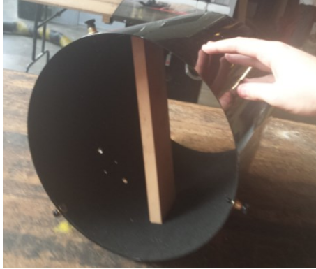
Figure 58. Our method of steadying the dew shield during manufacturing likely deformed the part.
