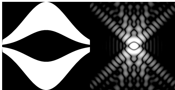
Figure 117. The Gaussian boomerang mask and its characteristic diffraction pattern, plotted on a nonlinear brightness scale.
