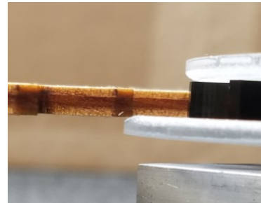
Figure 100. The tapering of the pinion lips, though subtle, effectively keeps the gear teeth from getting caught on the edge of the lips.
