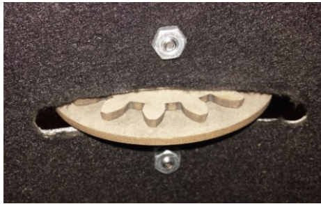
Figure 55. One of the mask-supporting lips of the virtual axis design, viewed from the interior of the dew shield.
