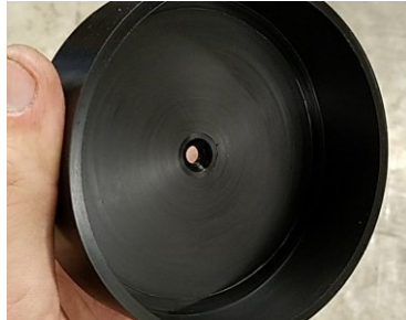
Figure 94. A newly machined axle cap. (Photo by Kevin Jantz.)
