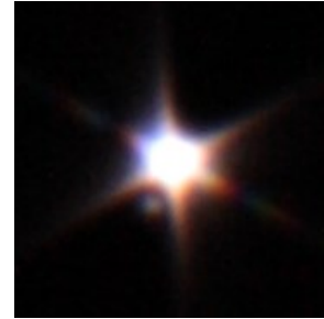
Figure 107. Rigel as seen through a prototype Gaussian donut mask, captured by Ray. (1.0-second exposure, ISO 800, f/10; captured with temperature below dew point in presence of high clouds).
