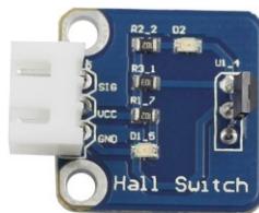
Figure 88. A Hall effect sensor breakout board (SunFounder, 2017). The sensor itself is the black component at the right side of the image.
