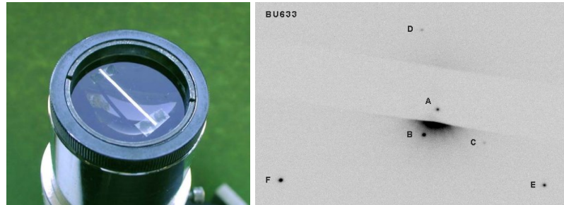
Figure 8. Left, an occulting strip affixed to a field lens (Daley, A Method of Measuring High Delta m Doubles, 2007); right, color-inverted image of \gamma Draconis captured with the occulting strip (Daley, A Method of Measuring High Delta m Doubles, 2007). Without attenuation, the light from star A would saturate the CCD sensors and hide other stars in the image.
