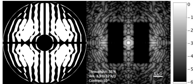
Figure 39. Left, an optimal pupil apodization for a version of SPICA with a four-legged spider and a 20-percent central obstruction. The design achieves a contrast ratio of 10^{-6} at working angles between 3.5 and 12 \lambda/D (Carlotti et al., 2011). Note the presence of free-standing islands. Right, the point spread function of this aperture (Carlotti et al., 2011).
