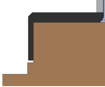
Figure 67. Section view of the axle cap's interface with the telescope. The axle cap is black; the telescope is brown. The depth of the cap is just less than the height of the upper part of the secondary mirror cylinder; meanwhile, the outer diameter of the cap is just shy of the diameter of the lower step of the secondary mirror cylinder.
