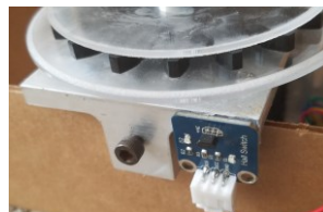
Figure 89. A Hall effect breakout board attached to the side of the motor bracket.
