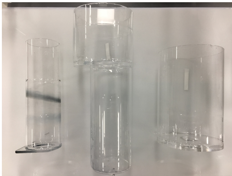
Figure 2. Different inner quartz tubes. The left tube is for supporting the middle tube with \text{Ø}120 \times 320 \text{ mm}^3 , the middle tube is for sample loading with \text{Ø}129 \times 300 \text{ mm}^3 (bottom side) and \text{Ø}172 \times 145 \text{ mm}^3 (top side), and the right tube is for sample collection with \text{Ø}180 \times 265 \text{ mm}^3 .
