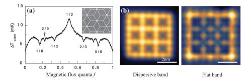
Figure 3. (a) Aharonov-Bohm cage in superconducting wire network. The superconducting transition width  $\Delta T$  shows a broad peak in the flat band limit f = 1/2, associated with the formation of decoupled compact localized states. Inset is an image of the dice lattice network [97]. (b) Selective imaging of dispersive and flat band states of an electronic Lieb lattice by changing the applied bias voltage and performing spatially resolved conductance measurements [98].
