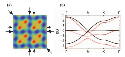
**Figure 4.** An optical Lieb lattice for cold atoms. (a) Lattice potential formed by five interfering standing waves (indicated by oppositely aligned arrows). Lattice sites lie at the potential minima in blue. (b) Band structure for shallow (red dashed lines) and deep (solid black lines) lattices computed in Ref. [119].
