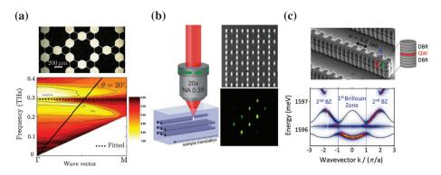
**Figure 5.** Examples of photonic flat bands: (a) Kagome lattice for terahertz spoof plasmons, displaying an omnidirectional minimum in the transmission at the flat band frequency (dashed line) [141]. (b) Femtosecond laser-written Lieb lattice waveguide arrays and an observed compact localized flat band state [143]. (c) Structured microcavity forming a 1D stub lattice and its photoluminescence spectrum revealing a middle flat band [144].
