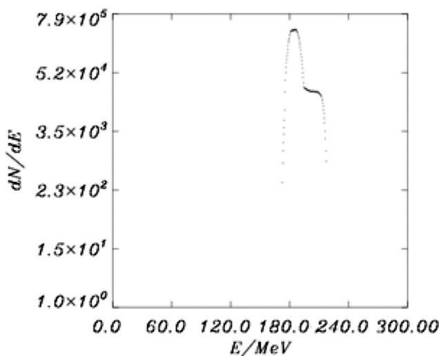
FIG. 8. Distribution function of protons in case of the acceleration of 80 MeV mono-energetic bunch by the factor of 2.5. Laser pulse with an intensity  $10^{21}$  W/cm<sup>2</sup>, duration 40 fs, and  $6 \mu\text{m}$  diameter irradiates Al<sup>+6</sup> target with ion density of  $10 n_{cr}$ , and thickness of  $5 \mu\text{m}$  in which the proton bunch with density  $n_p = 0.05 n_{cr}$  moves.
