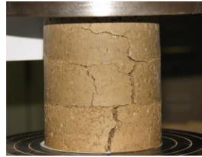
Figure 4. Failure pattern typical of brittle specimens.
