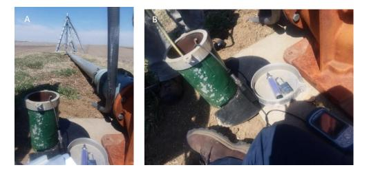
Figure 19 Shelter containing drop pipe with transducer cable showing the connection to the center pivot (A); same well with the water level being taken (B)
