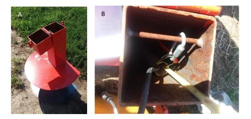
Figure 20 An alternate shelter for pressure transducer within a drop pipe (A) and water level being taken from similar installed shelter showing the PVC drop pipe (B)
