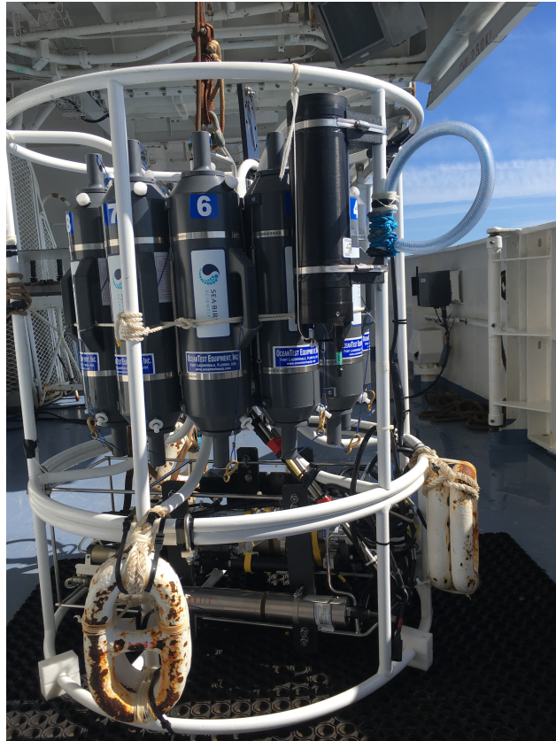
Figure 3.2: The CTD rosette with the SUNA nitrate sensor and battery pack.
