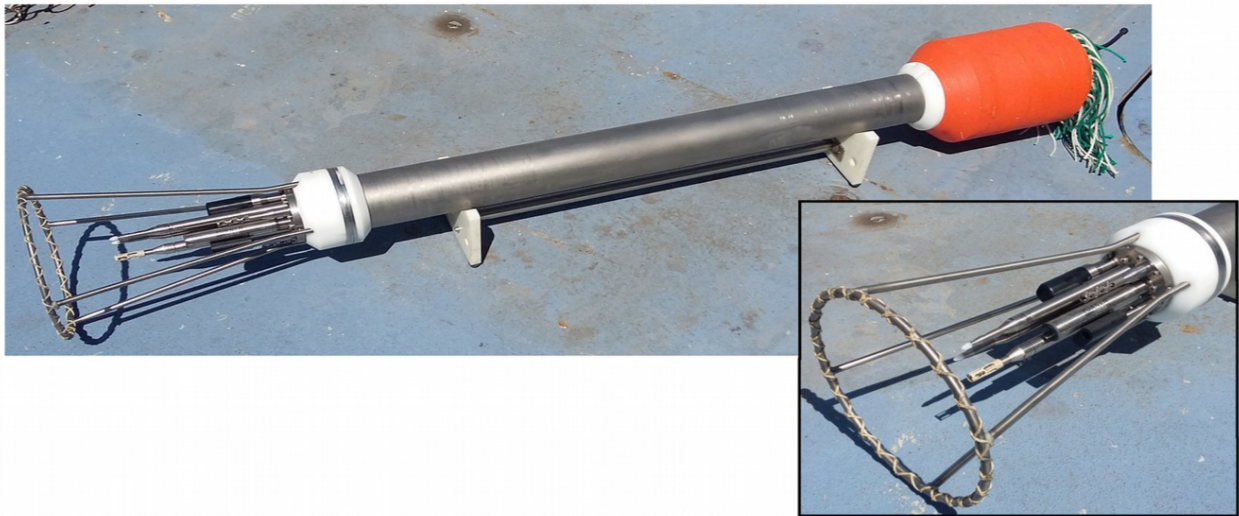
Figure 6.1: The MSS90L No. 069 used during the CALYPSO 2019 cruise. Insert shows the sensor head.
