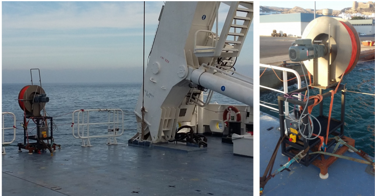
Figure 6.2: The winch set up at the stern of N/O Pourquoi Pas?
