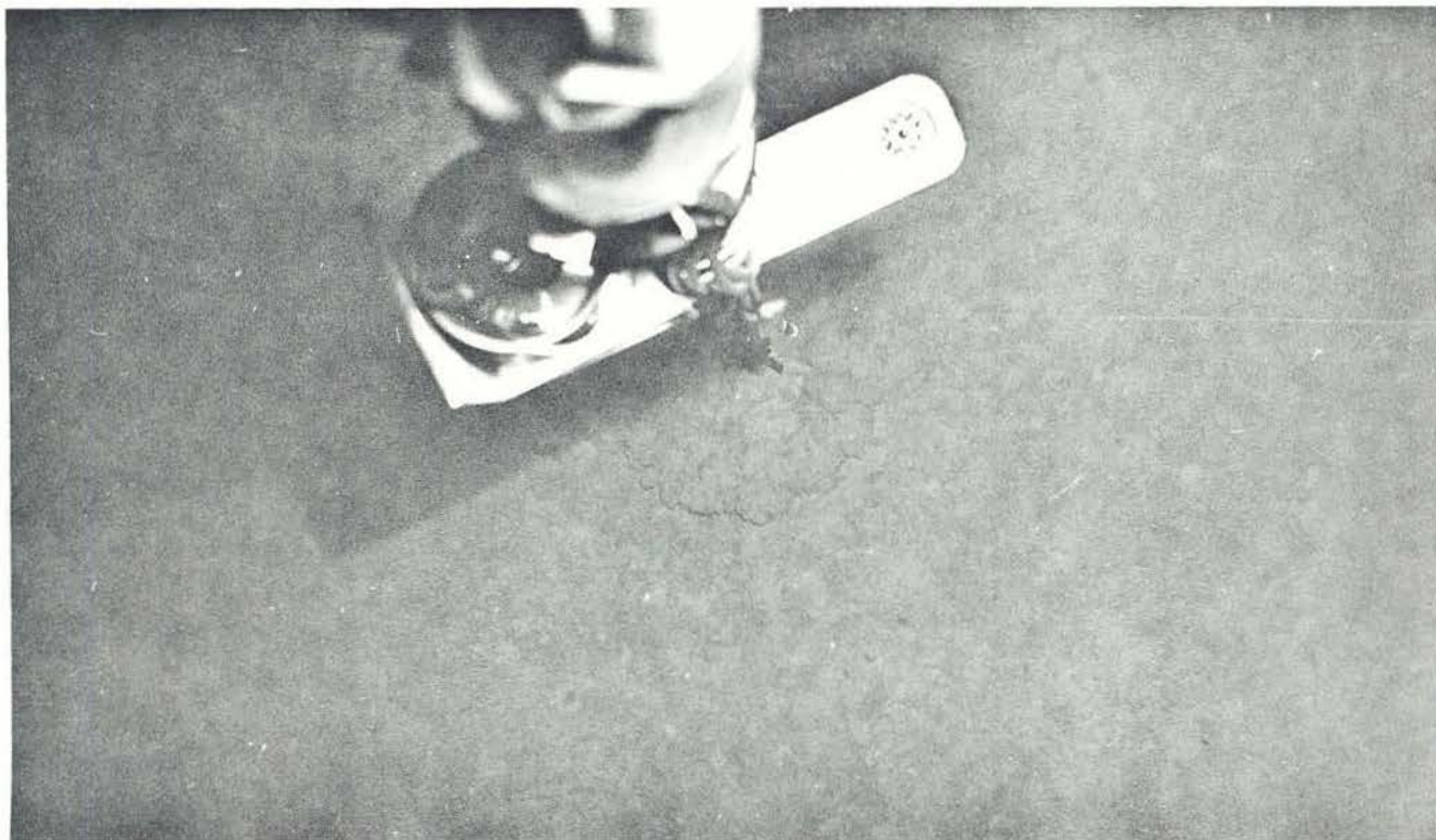
Figure 10. Penetration of the piston corer into the bottom on station 17. Note sediment cloud produced by the corer upon impact with the bottom. Penetration continued to about 60 cm from the corehead, burying the bracket arm and the other instruments mounted opposite the bracket arm. Photograph taken by the camera focused at 4.9 m (16 ft).
