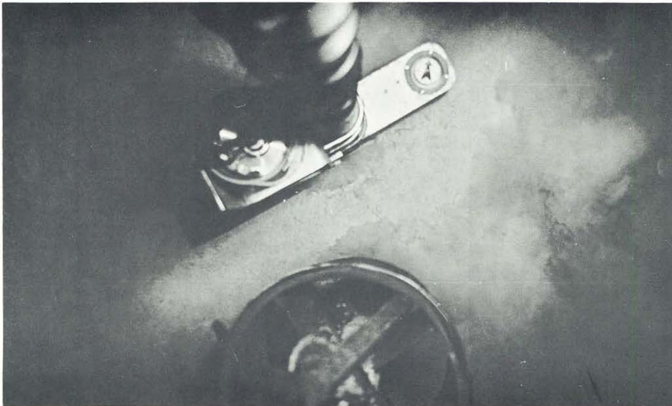
Figure 18. Pilot corer and piston corer in the bottom during station 14. Photograph taken by the camera focused at 4.9 m (16 ft).
