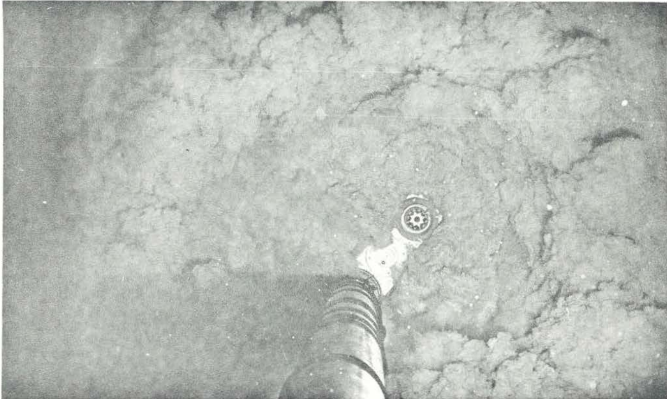
Figure 11. Penetration of the piston corer into the bottom on station 31. Penetration continued to about 90 cm from the corehead, burying the bracket arm. Photograph taken by the camera focused at 1.8 m (6 ft). The vertical deviation of the corer during penetration is 10^\circ , as recorded by the inclinometer.
