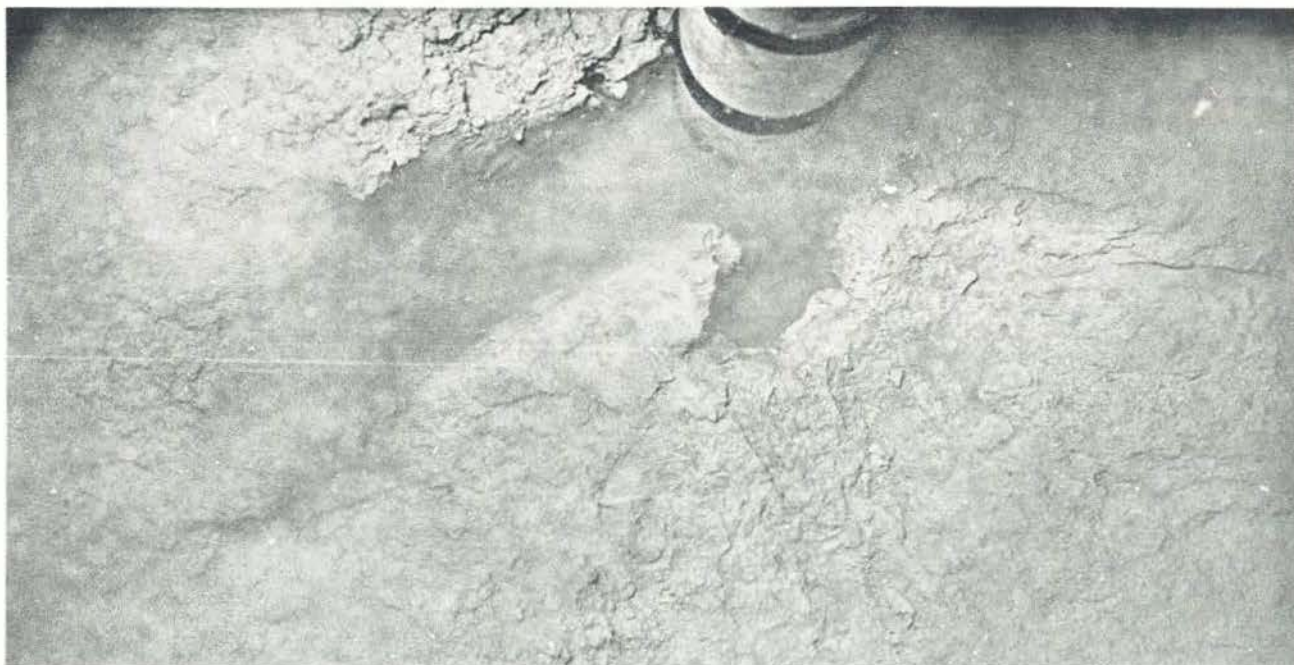
Figure 14. Portion of sediment mound surrounding core barrel on station 37. Rectangular hole to the left has been formed by the bracket arm. Photograph taken by the camera focused at 1.8 m (6 ft).
