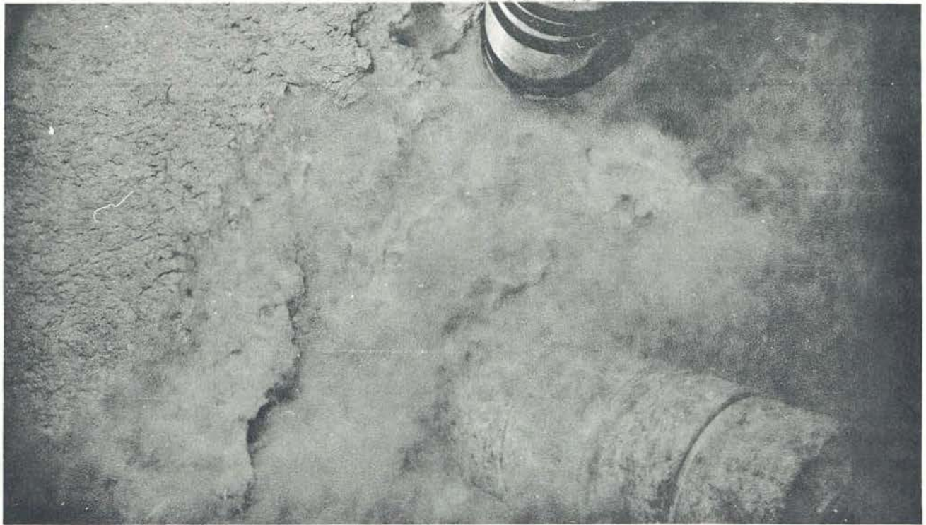
Figure 21. Pilot corer resting on its side near the piston corer on station 18, after swinging around the piston corer. Photograph taken by the camera focused at 1.8 m (6 ft).
