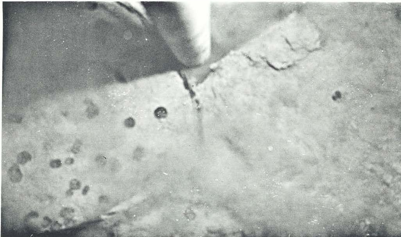
Figure 13. Small manganese nodules near the core barrel on station 2. Penetration has been completed here; figure 9 shows the corer in the process of penetration. These nodules have not been disturbed by the corer during penetration, as can be seen by comparing this photograph with figure 9. Note the cable lying on the bottom. Photograph taken by the camera focused at 4.9 m (16 ft).
