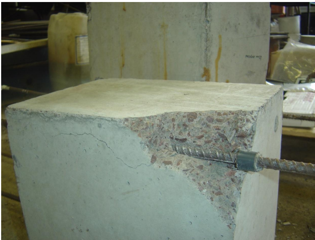
Figure 5.3: Splitting failure for corner bar location (specimen 10/2.5/BC/2)
