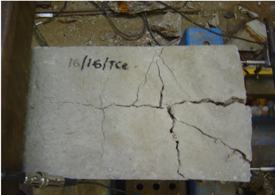
Figure 5.4: Splitting failure for centre bar location (specimen 16/1.6/TCe/2)
