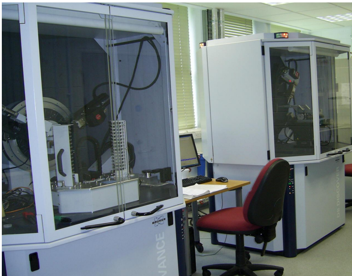
Figure 2.2: Bruker D8 Advance (left) and D8 Discover diffractometers used in this work.
