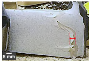
Figure 6 Spallation of the left-half straight blister.
