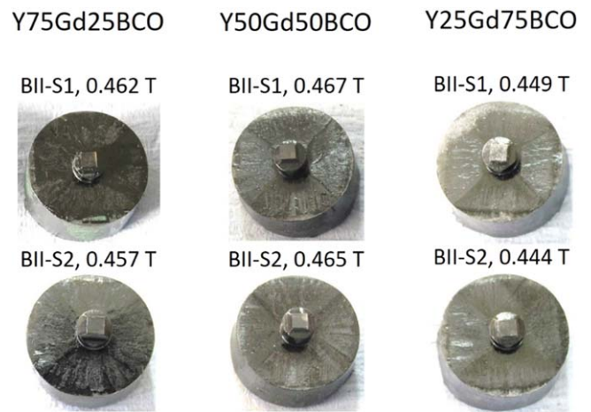
Figure 9. Second set of samples, 16 mm in diameter, fabricated using faster heating profiles.
