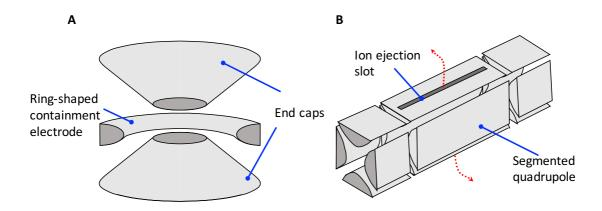
*Figure 1-VI.* Ion Trap Layouts. *A*: Three-dimensional (Ring) Ion Trap. *B*: Twodimensional (Linear) Ion Trap with hyperbolic electrodes (modern designs are typically segmented to optimise the distribution of the radiofrequency field).
