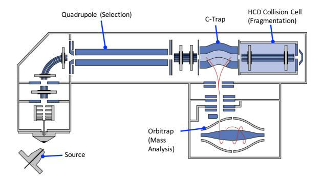
*Figure 1-XIII.* Thermo Fisher *Q*-Exactive Schematic. Adapted from Thermo Fisher product literature.
