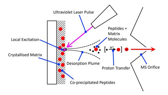
*Figure 1-III. MALDI Ionisation of Peptides from a Photoabsorbant Matrix. Adapted from de Hoffmann, E., and Stroobant, V., 2007 (60).*
