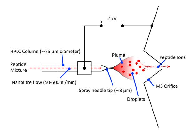
*Figure 1-II. Electrospray Ionisation of Peptides from Nano-Flow HPLC Column. Adapted from Steen, H., and Mann, M., 2004 (43).*
