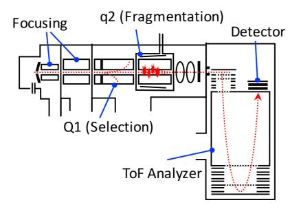
*Figure 1-XI. ABSciex TripleTOF 5600 Quadrupole-ToF Schematic. Based on ABSciex product literature.*
