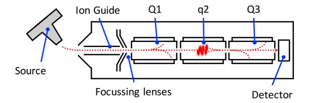
*Figure 1-X. Triple Quadrupole Schematic. In*  $MS^2$  *mode, ions are selected in Q1 (fixed filter), fragmented in q2 and scanned out to the detector (scanning filter) in Q3.*
