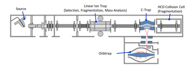
*Figure 1-XII.* Thermo Fisher LTQ-Orbitrap XL Schematic. Adapted from Thermo Fisher product literature.
