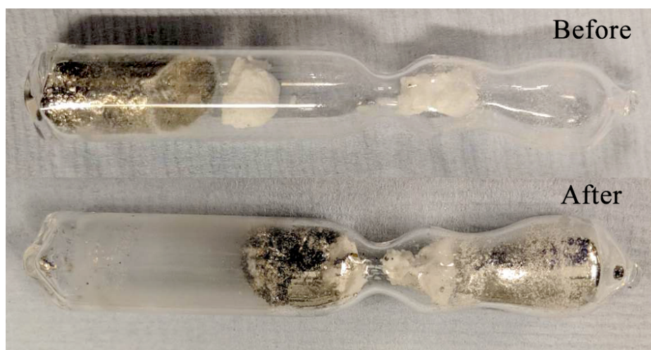
Fig. 3.4 Pictures showing an ampoule enclosing crystal-containing Sn flux before (upper panel) and after (lower panel) centrifugation.
