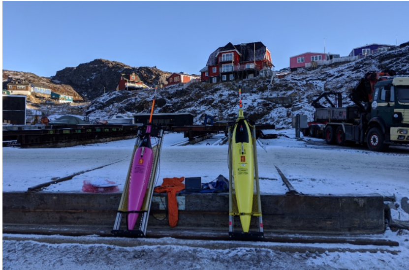
Figure 7.1: Seagliders undergoing sim dives.
