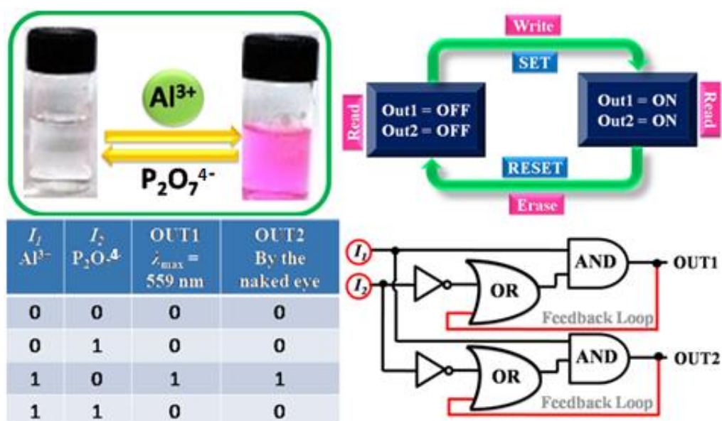
Fig. 8. Truth table, sequential logic circuits displaying memory units with two inputs ( I_1 , \text{Al}^{3+} and I_2 , \text{P}_2\text{O}_7^{4-} ) and two outputs and schematic representation of the reversible logic operations for memory element holding “write-read-erase-read” functions.
