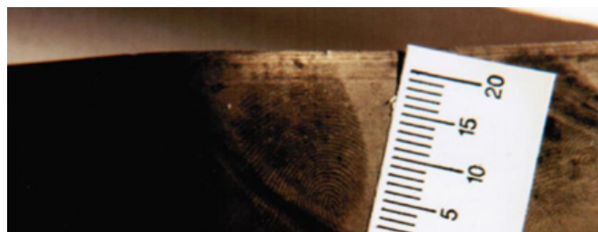
Figure 10 Metal light found directly above origin of fire, the fingerprint is 'baked on'. 38
