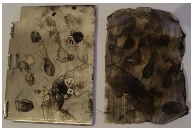
Figure 8 Left is the metal plate once the dried latex has been removed. Right, is once the liquid latex has dried. 27
