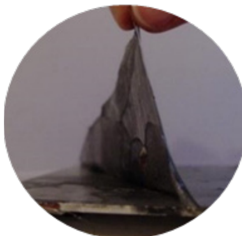
Figure 7 Peeling off dried liquid latex and the soot that has adhered to it. 27
