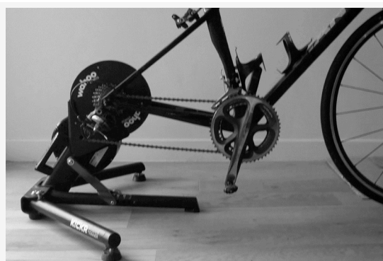
Figure 1. a) The attachment of the KICKR to the drivetrain of a bicycle; & b) Superior view. 1: Flywheel; 2: Belt drive; 3: Cassette.
