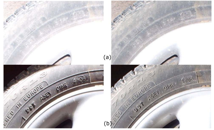
Fig. 3. Tyre sidewall with code printed. Same tyre and position with only changing illumination source position. Light angles (a) orthogonal or frontal (b) oblique w.r.t the plane of the sidewall. The breakdown of the code is: DOT (Department of Transport USA approved), A5 (manufacturing plant), EY (tyre size, manufacturer specific), 018R (manufacturer-specific batch number) and 4808 (date of manufacture in WWYY format) [16]–[18].
