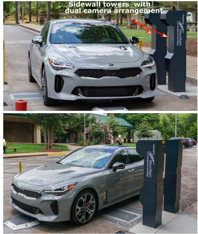
Fig. 13. Sidewall text reader with dual camera/light housing towers in operation (courtesy CNET.com).
