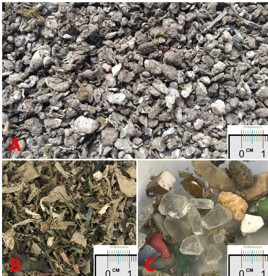
Figure 3.6: Photographs of trommel fines after manual separation; A: trommel fines (<2mm) for grinding after manual separation of inorganics and plastics; B: manually separated plastics and textiles; C: manually separated glasses and large stones (inorganics)
