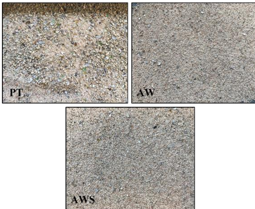
Figure 5.20: Reactor contents at the end of experiments after carbon burn off for dry and wet physically pre-treated trommel fine samples
