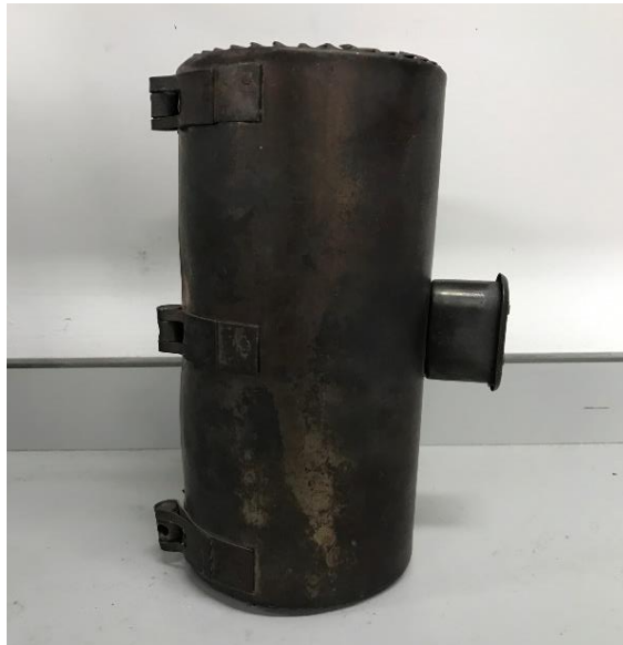
Figure 3.18: Original reactor band heater
