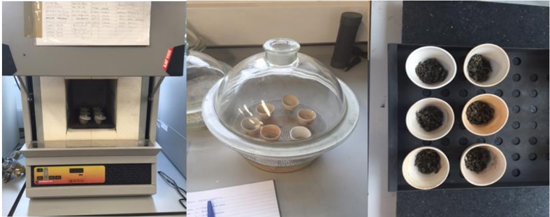
Figure 3.10: Carbolite AAF1100 furnace, desiccator and crucibles used for proximate analysis during this research (Source: EBRI Industrial Laboratory 02)
