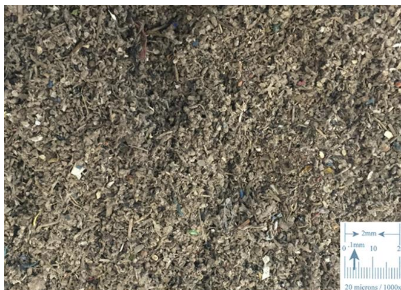
Figure 4.6: Photograph of prepared trommel fines fraction (0.5 – 2 mm size range) for fast pyrolysis
