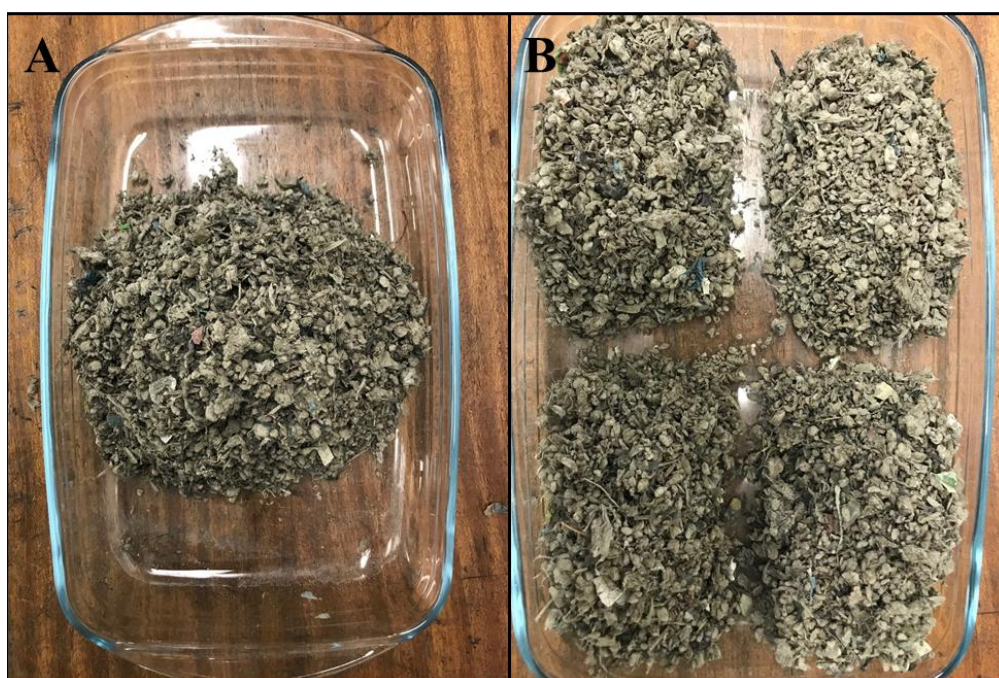
Figure 3.4: Photographs of trommel fines sampling; A: coning of trommel fines; B: quartering of trommel fines
