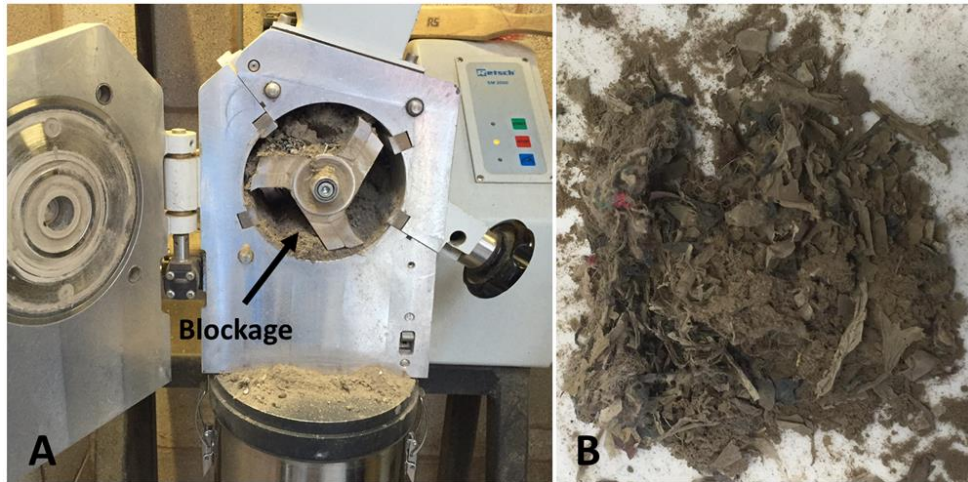
Figure 3.5: Retsch SM 2000 grinding mill: - A: blockage to mill blade caused by inorganics and plastics. B: inorganics and plastics removed from grinding mill (Source: EBRI Biomass storage room)
