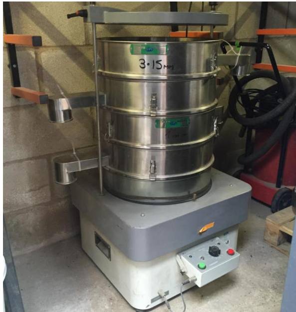
Figure 3.2: Powermatic sieve shaker with 0-3.5 mm sieve stack (Source: EBRI Biomass storage room)
