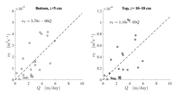
Figure 3.31 Correlation between turbulent viscosity and mussels' collective pumping rate. Dashed lines and equations in the figure represent linear regression of  $v_T = \gamma Q$ .
