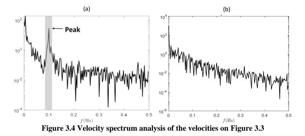
(a) is the velocity spectrum of the abnormal case and (b) is the velocity spectrum of the normal case.
