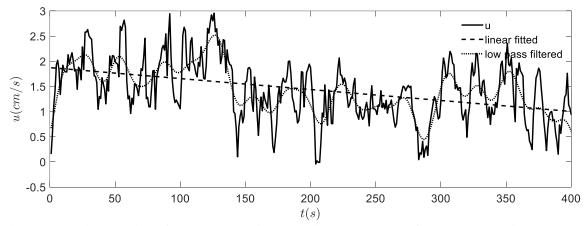
Figure 3.5 Time series of the streamwise velocity at z = 5 cm from data set AW55-0023. The dotted line represents the lowpass filtered (= 50 s) velocity signal. The solid line is the horizontal velocity, where the dashed line and the dotted line are lowpass filtered and linear regressed velocities. The sample rate is 1Hz.
