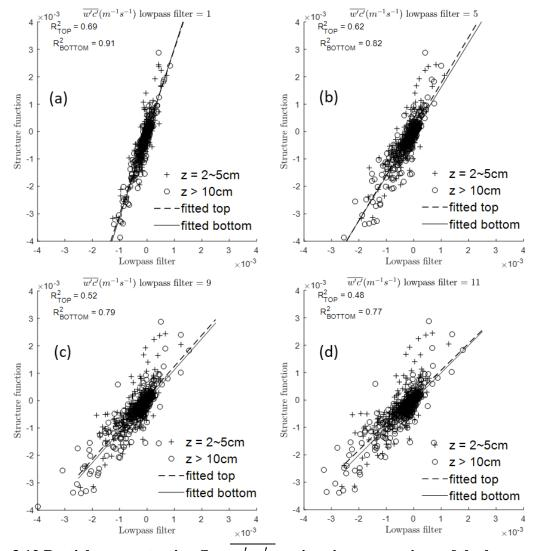
Figure 3.12 Particle concentration flux w' c' estimation comparison of the lowpass filter method and the structure function method.
