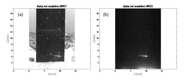
Figure 2.3 Particle images captured during daytime and night. The comparison shows that the background board shows excellent performance of blocking the sunlight.
