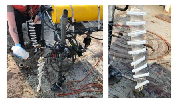
Figure 2.11 The membrane tube attached in the UWMPIV frame
