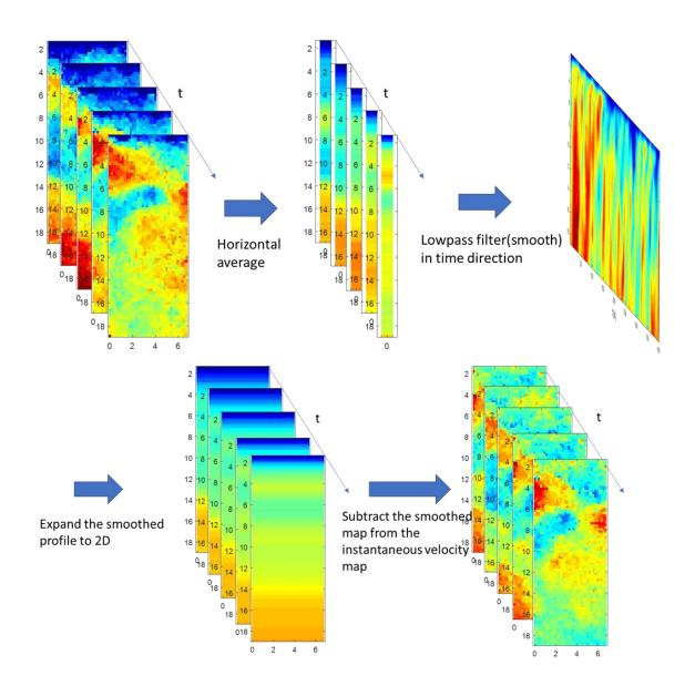
Figure 3.7 Lowpass method data processing steps
