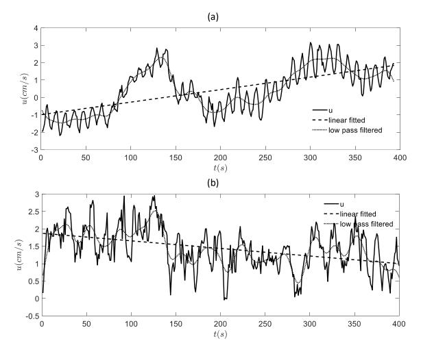
Figure 3.3 Time series of the streamwise velocity at z = 5cm. (a) A typical Time series of the streamwise velocity at z = 5 cm from data set. The dotted line represents the lowpass filtered (= 50 s) velocity signal. The solid line is the horizontal velocity, where the dashed line and the dotted line are lowpass filtered and linear regressed velocities. (b) is a case with normal time series streamwise velocity
