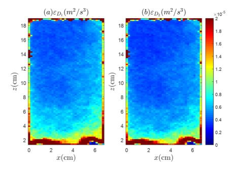
Figure 3.13 (a) TKE dissipation rate calculated by Hinze's direct method. (b) TKE dissipation rate calculated by Doron's direct method. The dataset is AW55-0023.
