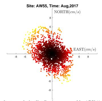
Figure 3.1 Near bottom velocity distribution measured by ADV (Acoustic Doppler Velocimeter) on the site of AW55 in August 2017. The ADV sample volume was located 25cm above the lake bottom which is close to the PIV measurement ROI (from 0cm to 20cm above the bottom), every data points represents a
