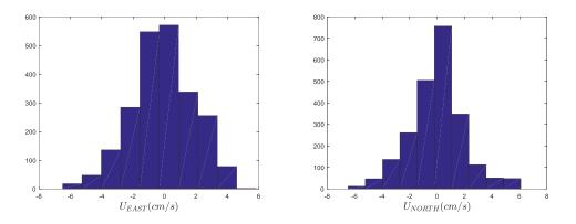
Figure 2.9 Histogram of the velocity measured by an ADV at the height of 25cm above the lake bottom.
