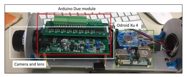
Figure 2.4 Inside the Camera-Computer unit.
