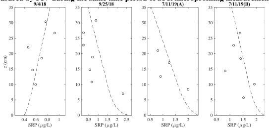
Figure 4.8 Profiles of SRP from microprofiler measurement (circles) and from model solution (solid line), with the SRP flux  $F_{DP}$ , bottom concentration  $C_{DP0}$  and the diffusivity D(z) all estimated with nonlinear fitting, since PIV data were not available during the microprofiling measurements.
