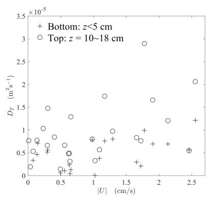
Figure 3.27 Comparison of the mean velocity and the turbulent diffusivity
