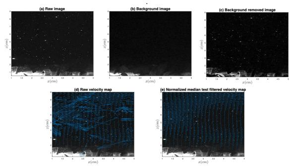
Figure 2.12 An example of PIV pre-process, interrogation result and post-process (adaptive median test) result.
