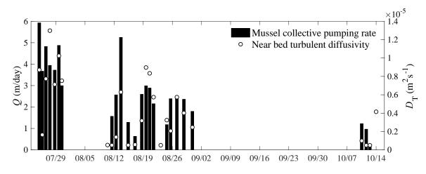
Figure 3.29 Time series of estimate mussel collective pumping rate (converted to m/day) and near-bed diffusivity
