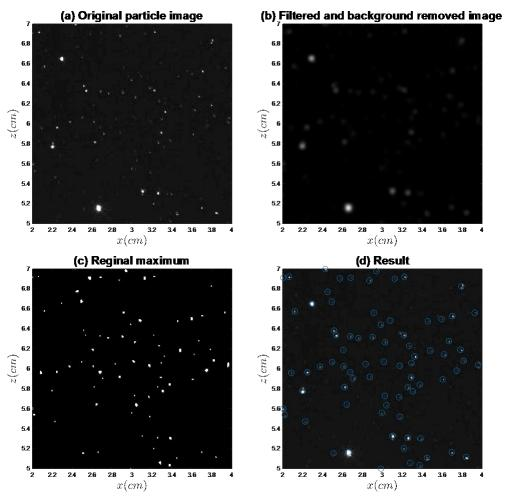
Figure 2.13 An example that illustrates the particle identification algorithm. (a) Raw PIV image, (b) image after background removing and smoothing, (c) binary image generated by regional maximum finding, (d) particles identified are marked with circles.
