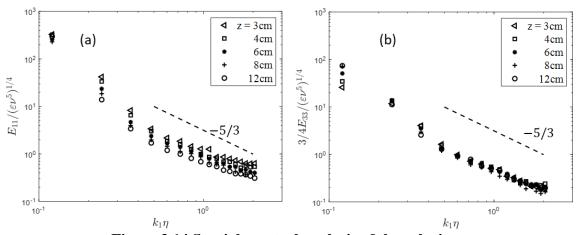
Figure 3.14 Spatial spectral analysis of the velocity. (a) is the streamwise horizontal velocity spectrum  $E_{11}$ , (b) is the streamwise vertical velocity spectrum  $E_{33}$ .
