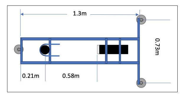
Figure 2.1 Structural configuration of the Underwater PIV system.
