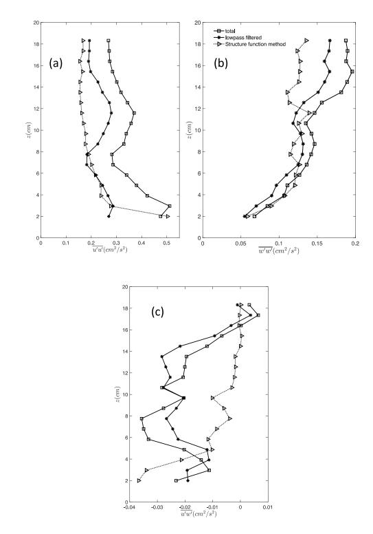
Figure 3.9 (a)(b) Reynolds normal stress and (c) Reynolds shear stress by second-order structure function method and the lowpass filter method.
