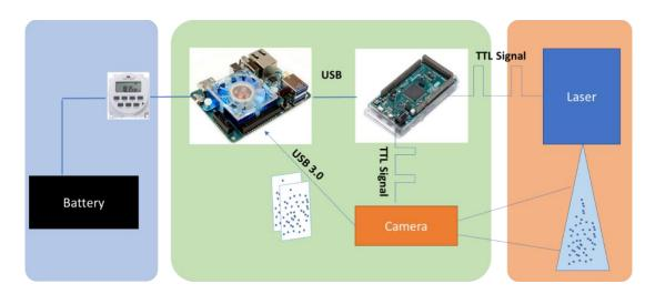
Figure 2.5 UW-PIV synchronization signal flow chart
