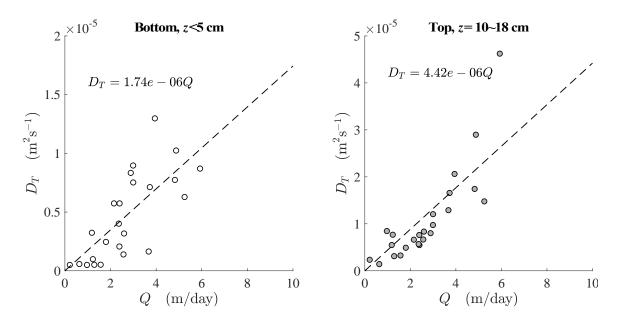
Figure 3.30 Correlation between turbulent diffusivity and mussels' collective pumping rate. Dashed lines and equations in the figure represent linear regression of  $D_T = \gamma Q$ .
