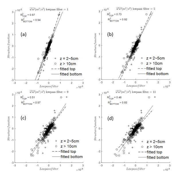
Figure 3.11 Reynolds shear stress comparison of the lowpass filter method and the structure function method.
