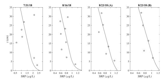
Figure 4.7 Profiles of SRP from microprofiler measurement (circles) and from model solution (solid line), with the SRP flux  $F_{DP}$  and bottom concentration  $C_{DP0}$  estimated with nonlinear fitting. Distribution of diffusivity D(z) is modeled with average diffusivity measured by PIV during the same time period of SPR microprofiling measurements.
