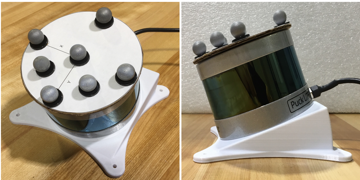
Figure 2.17 VICON pearls on LiDAR.
