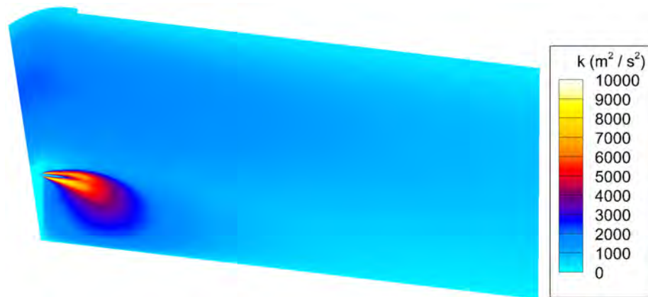
Figure 3.19 Transport of k within the injection for inflow k = 1000 \text{ m}^2/\text{s}^2
