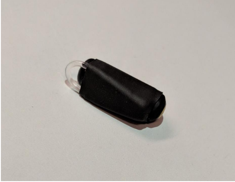
Figure 2. Acoustic transmitters were modified with a loop attachment site through the use of 50lb monofilament, electrical tape (3M Scotch \frac{3}{4} "), Loctite Ultra Gel (Henkel Corporation, Westlake, Ohio), and shrink wrap (HS515-1.22M – Heatshrink, 12 mm).
