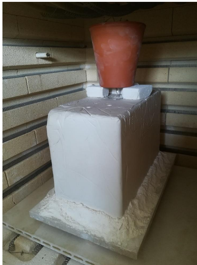
Figure 5.2: Prepared mould on kiln shelf within the kiln
