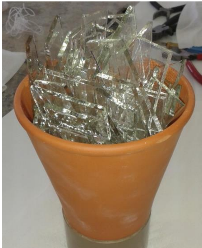
Figure 5.1: Crucible (unglazed flower pot) filled with pieces of Spectrum glass
