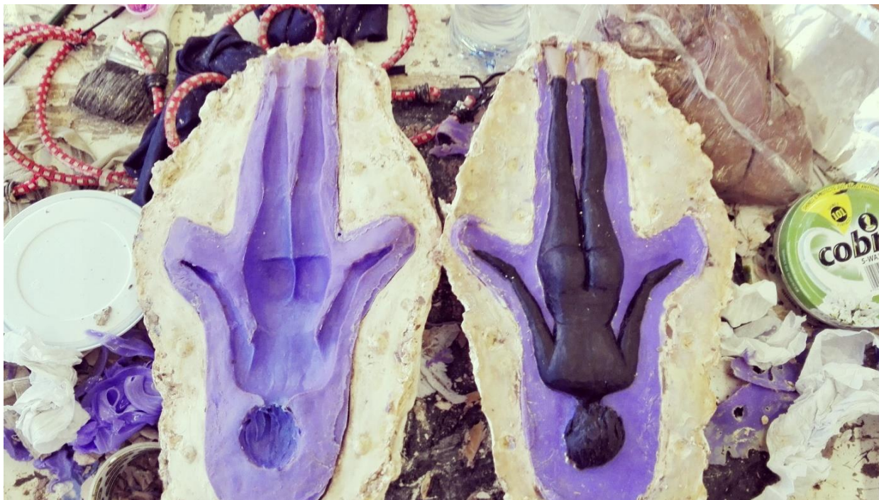
Figure 4.6: The demoulding of the Serendipity I wax sculpture showing the two-piece rubber mould and plaster of Paris rigid support 'cap'.
