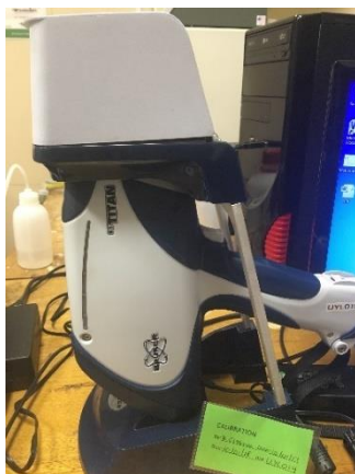
Figure 3.5: A photo of the handheld energy dispersive X-ray fluorescence (Bruker s1-TITAN Analyzer) instrument.
