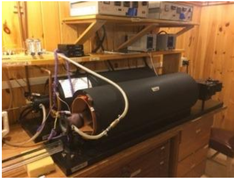
Figure 8. The ASC TD-48SC thermal specimen demagnetizer in Michigan Tech's Earth Magnetism Laboratory.
