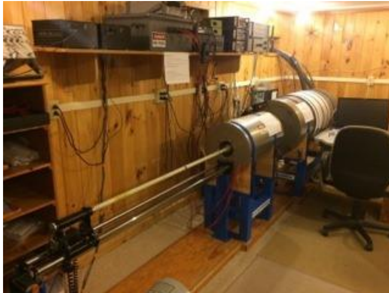
Figure 7. The 2G Enterprise 760-R superconducting rock magnetometer in Michigan Tech's Earth Magnetism Laboratory.
