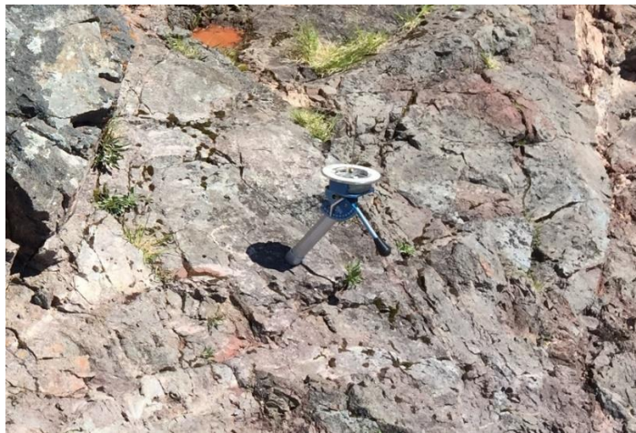
Figure 6. The Pomeroy Orienting fixture with a Brunton compass used to orient the core samples.
