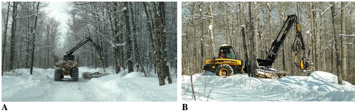
Figure 5. A showing a forwarder as part of a cut to length system and B showing a harvester (PONSEE bear)
