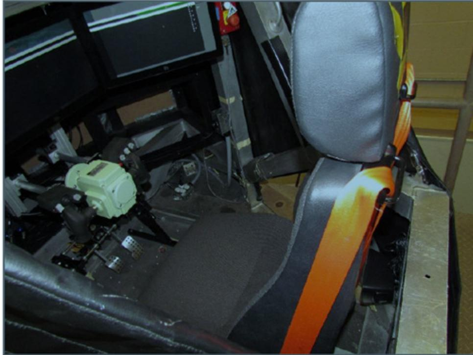
*Figure 5.1: Crewstation Configuration with Ultra MSI Driving Gunner Yoke*
