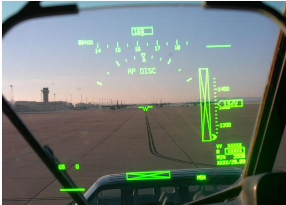
*Figure 2.2: Example of Heads Up Display (HUD). Image source: <https://www.dyess.af.mil/News/Article-Display/Article/269558/a-new-hercules-for-the-21st-century/>.*
