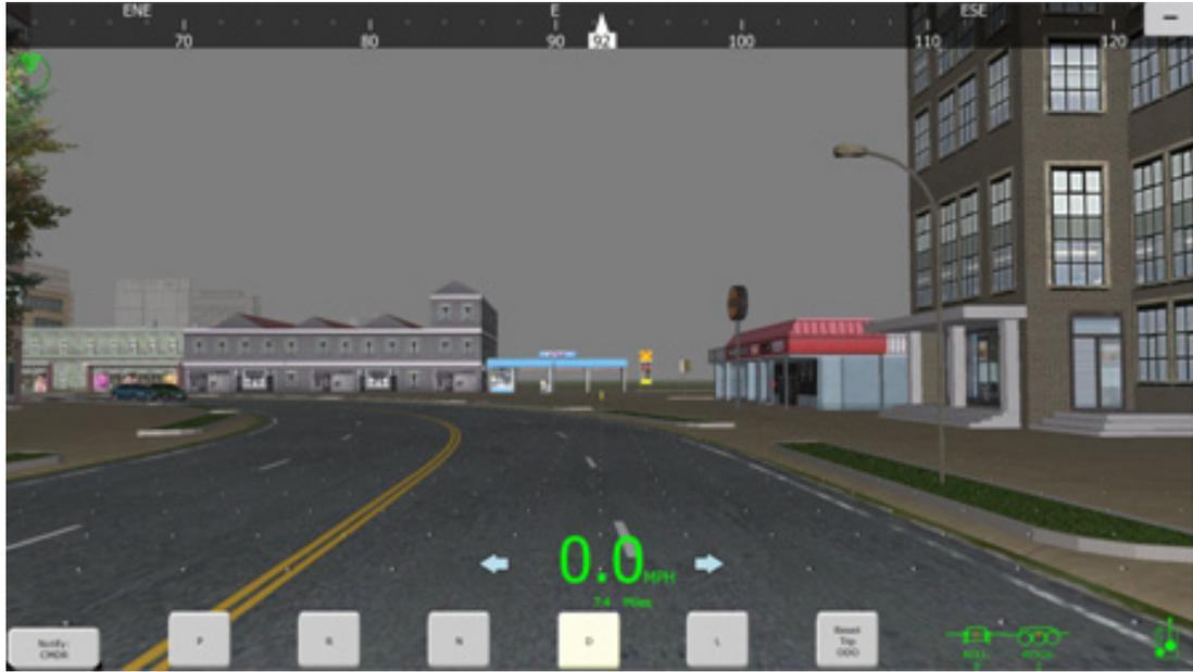
Figure 3.4: Urban route with Optic Flow Driving aid presented as dots at ground level
