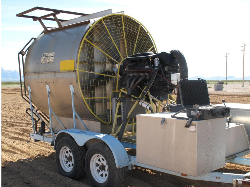
Figure 7.3: Blown Air Dust and Sand System (BADSS).
