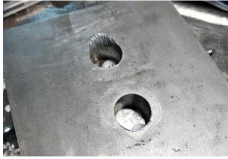
Figure 20. Deformation on one edge of a plug due to the friction between it and the cable passing through it.
