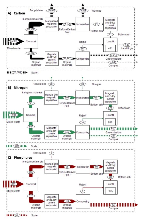
**Figure 3.1.** Flows of C (Figure 3.1.A), N (Figure 3.1.B) and P (Figure 3.1.C) in the Cantabrian mechanical biological treatment plant (ton·year<sup>-1</sup>). Estimation performed with the data from the Cantabrian waste management plan<sup>2</sup> and the elemental composition of the waste components provided by the EASETECH (Environmental Assessment System for Environmental Technologies) 2.3.6 software.<sup>3</sup>
