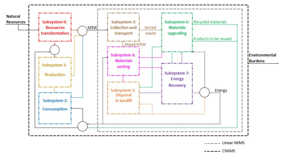
Figure 3.1.3. Configuration and boundaries of a CIWMSs
