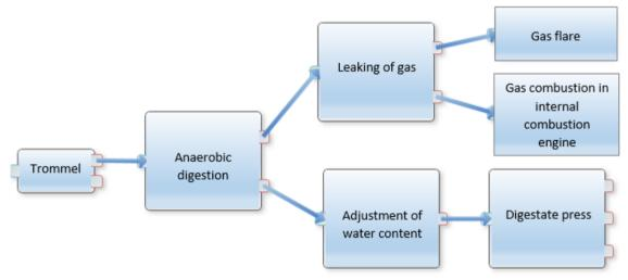
Figure S3. Sub-models of the anaerobic digestion unit process
