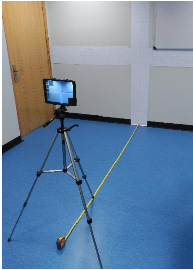
514 Fig. 11. Variation of the angular fields of view of the device real camera depending on the working 515 distance to the target.
