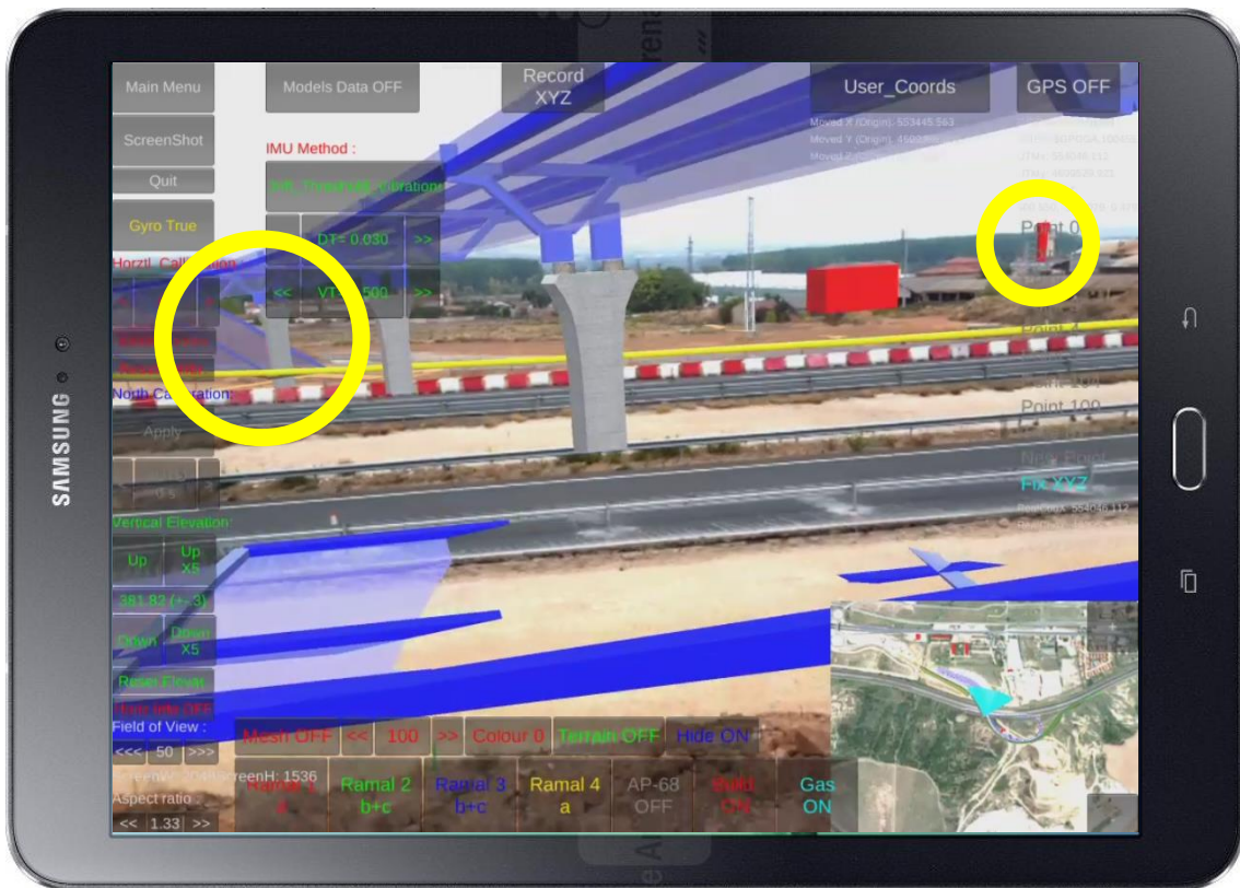
488 489 Fig. 10. Misalignments in the scene between the virtual and real objects.
