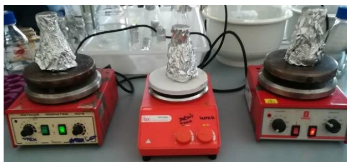
Figure 21 - The extracts mixing in individual stirrers at room temperature. The extracts were wrapped in aluminum foil to prevent pigment degradation.
