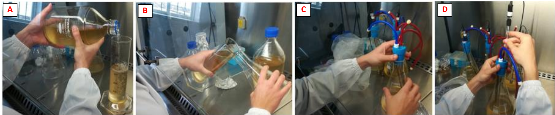
Figure 13 – The different stages of preparation for an Algem incubation. A,B – Dilution of Necton’s culture and inoculation inside a laminar flow chamber. C,D- Setup of Algem lid which is connected to the CO 2 injection system, air entrance and exit, as well as a pH probe. From here, the Erlenmeyers were placed inside each chamber to start the experiment.
