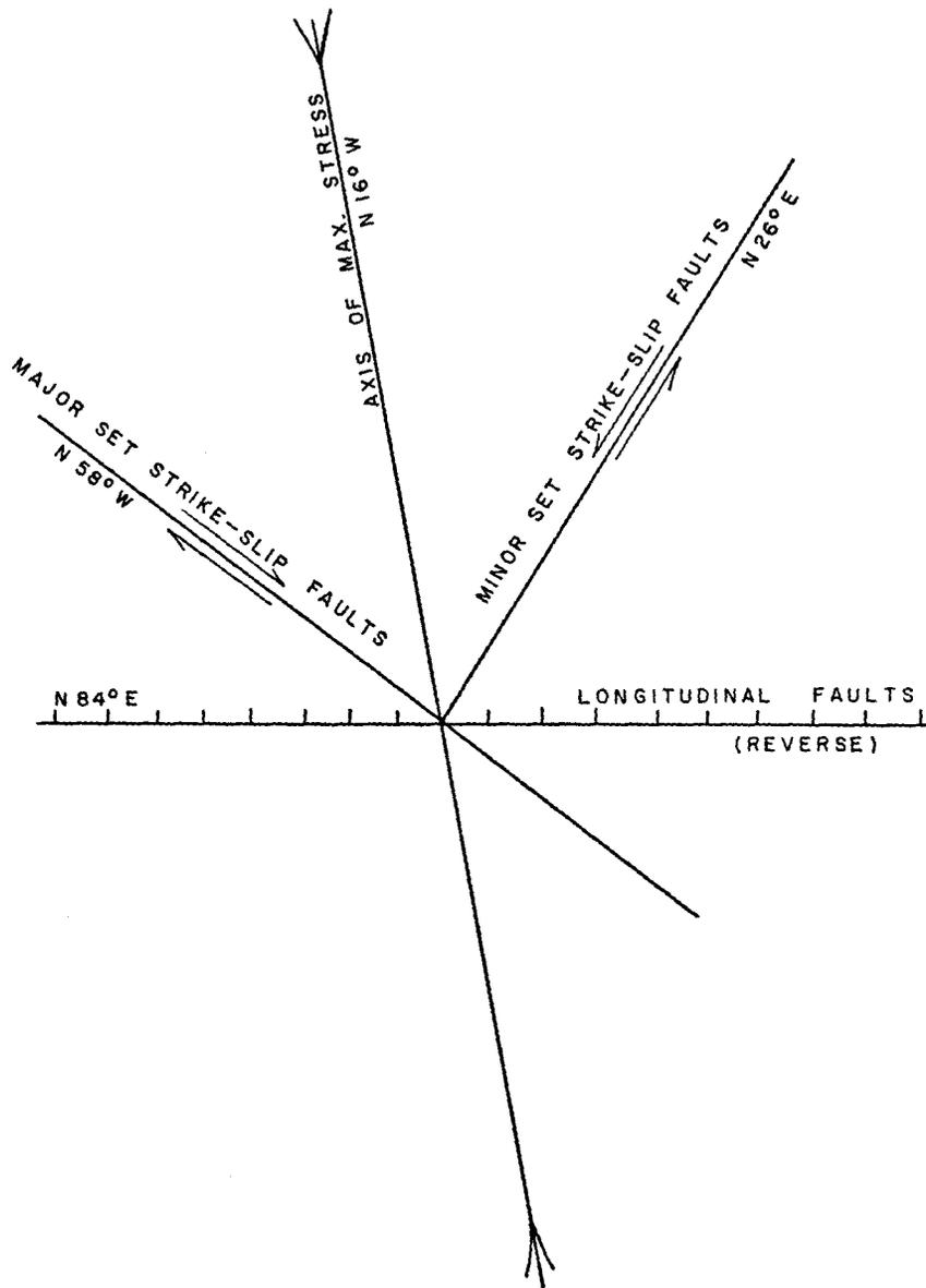
FIG.—16 RELATION OF AXIS OF MAXIMUM COMPRESSION TO AVERAGE TRENDS OF FAULT SETS IN PART OF COCINAS TROUGH
