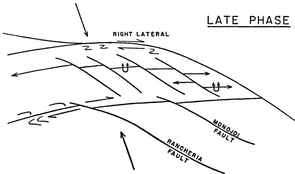
FIG.—17 GENESIS OF COCINAS STRUCTURAL PATTERNS
