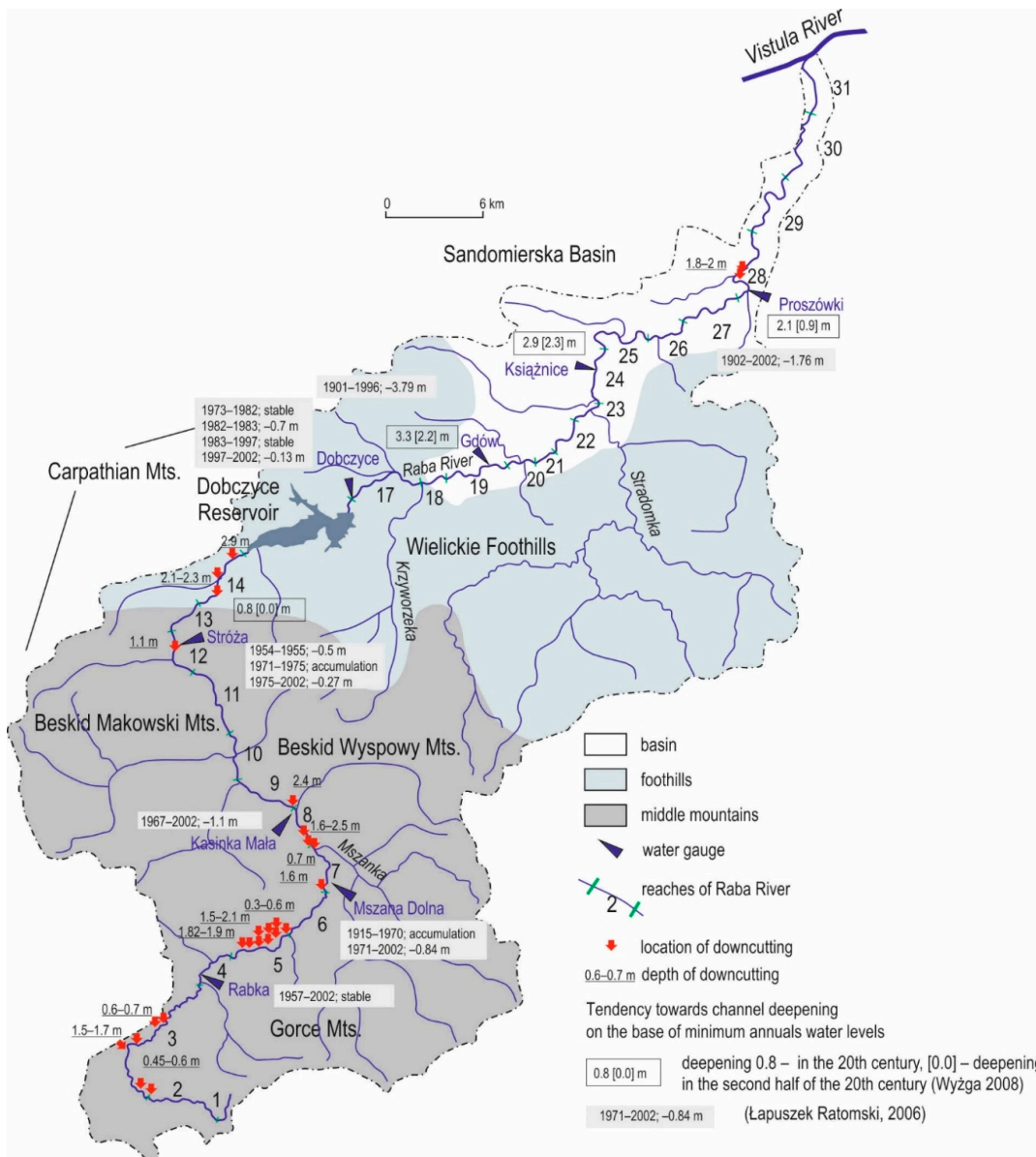
Figure 2. Location and intensities of downcutting in the Raba river channel.
