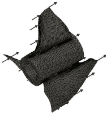
Figure 5 Boundary conditions and loads for the finite element analysis
