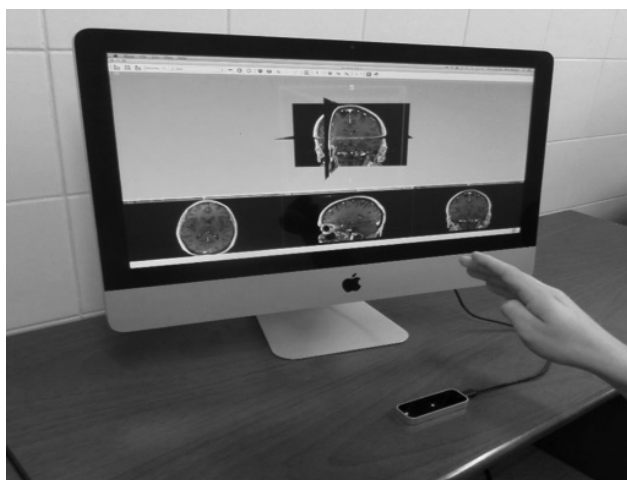
Figure 10 The movement of the planes is done by moving the hand over the physical space defined by the Leap Motion
