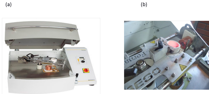
Figure 3 (a) BEGO induction furnace in argon atmosphere. (b) Actual photograph of the furnace arm.
