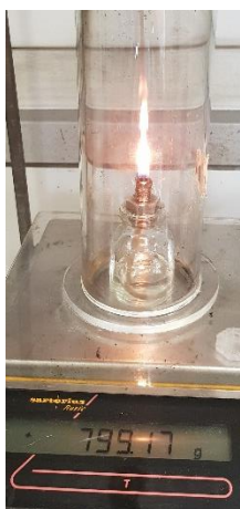
Figure B3. Non-premixed flames: fuel flow rate measurement (a) and fuel flow rate (b)
