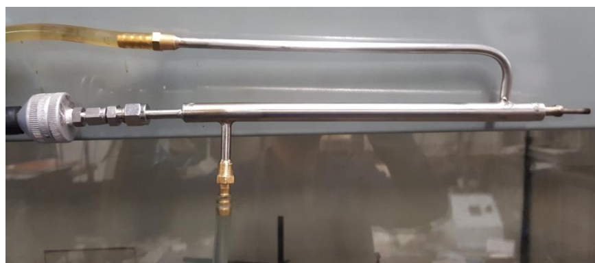
Figure C1. Stainless steel cylindrical case for sampling in diesel engine (a). Stainless steel mesh (b). Mesh with samples (c). Detail of mesh shaken (d)
