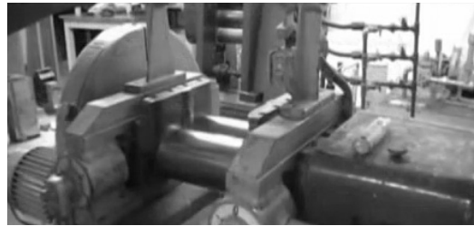
b) Types of open roll mills used for mixing
