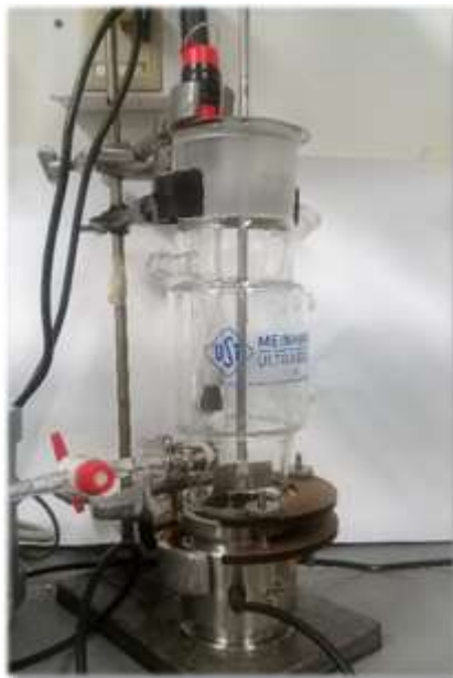
Figure 9. Fenton/Ultrasound/UV reactor Setup
