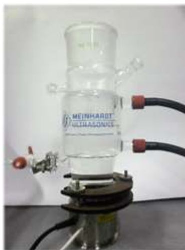
Figure 6. Glass reactor with Cooling Jacket
