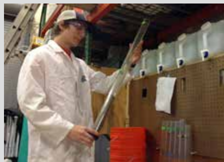
We used controlled column studies to explore how different soil gradients, depths, and amendments perform with respect to phosphorus removal from typical urban stormwater runoff. Column studies are a quick, efficient way to test the performance of a wide range of filter media.
