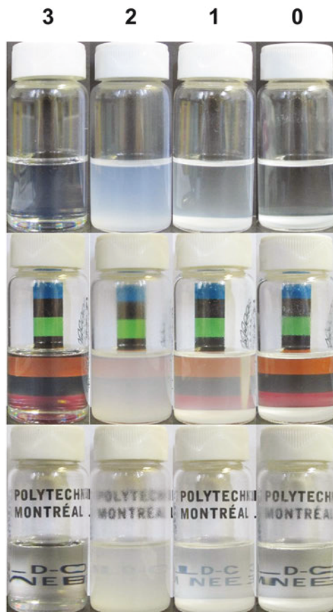
Fig. 2 – Dispersibility scale for sedimentation tests. From left to right, and from the best to the worst, 4 levels of dispersion were observed: 3-good, 2-partial, 1-weak, and 0-none. Pictures were taken on different backgrounds (from top to bottom) to help with the evaluation. Solvents presented here are from left to right: dimethylsulfoxide, N,N-dimethylformamide, 1-propanol, and 1,4-dioxane.
