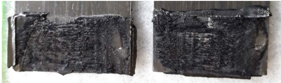
(b) Mostly cohesive failure in a sample welded for 90 s
