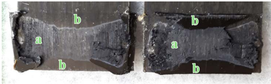
(a) Cohesive failure with a thinner section in the middle [a] and adhesive failure on the sides [b] in a sample welded for 70 s
