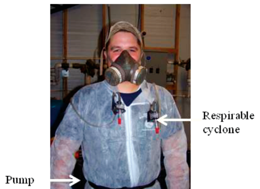
Figure 2. Two respirable cyclones were worn by each worker. Each cyclone was connected to a pump enclosed in a noise-reducing cover. Color version available in the online PDF.
