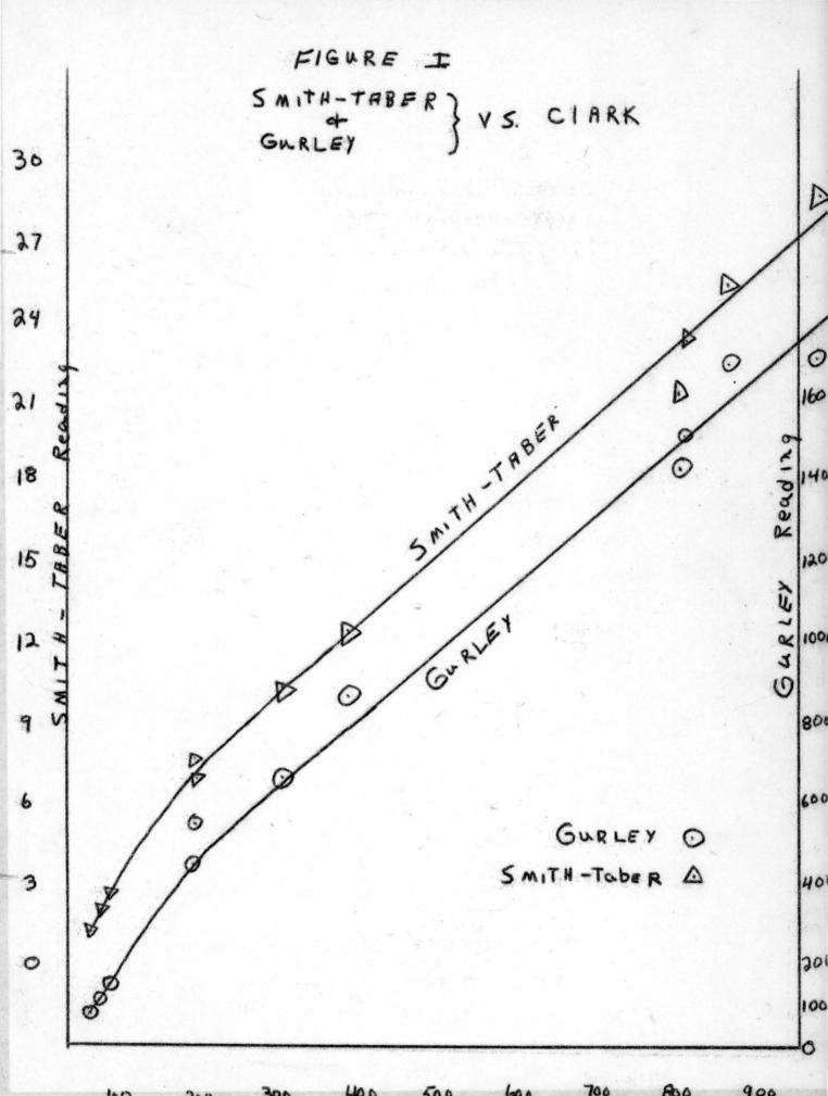
Referring again to the table, it is apparent that in the higher ranges, the readings of the different instruments vary by some integer. That is, the Gurley reading is about twice that of the Clark and the Clark reading is approximately 30 times as large as the Smith-Taber.
