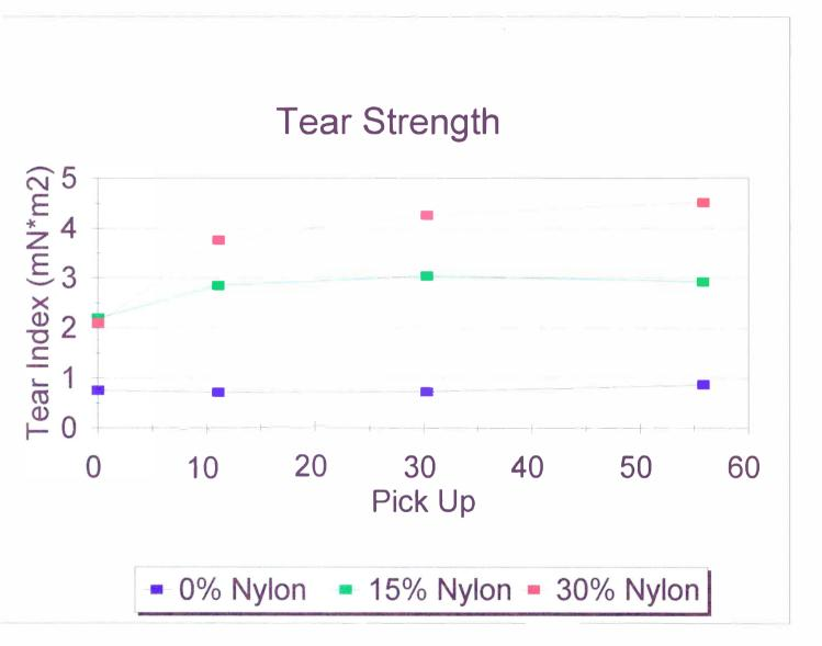
By observing the tear index graph on the previous page, it can be seen that the tear index increased proportionally as nylon was added to the furnish. A 15% increase in nylon addition contributed to a 100% increase in tear strength. This result was expected, since fiber length is the principle factor affecting tear strength.
