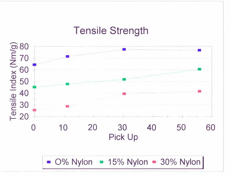
By viewing the graph showing the tensile index results, it can be seen that the tensile index linearly decreases as the nylon level is raised. These results were expected, and can best be described by analyzing Page's equation:
