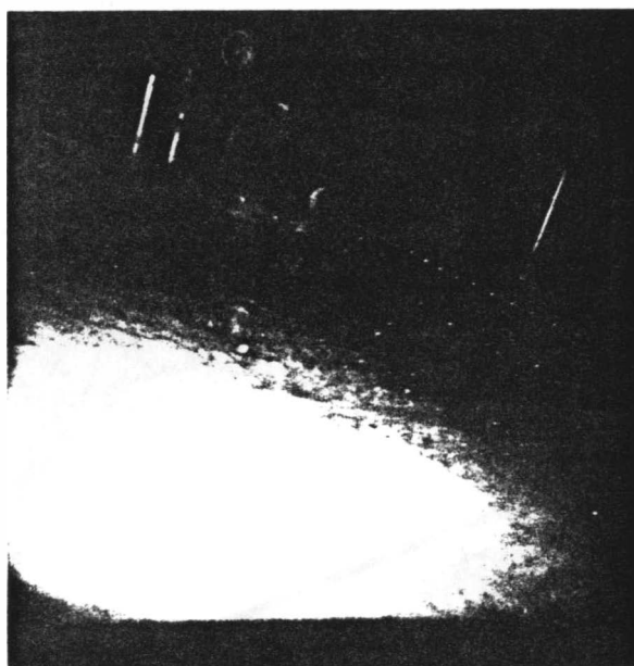
Figure 22. Stock Appearance with Formation Shower at Normal Consistency
