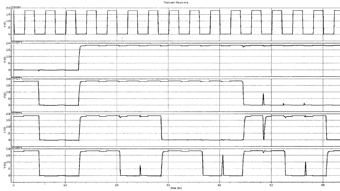
Figure 5.15: Simulation Waveforms for the RALUT, from Top to Bottom: Clock Signal, Output Line 3, 2, 1, and 0
